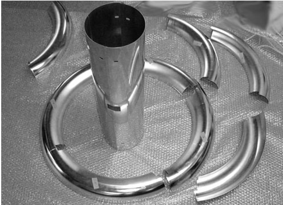
Figure 3.4: Plasma control electrodes before the installation.
