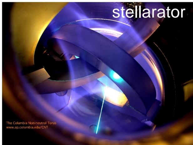
Steady-state closed magnetic surfaces are generated by interlocked current coils
