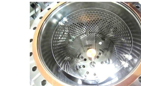
Segmented electrodes in prototype dipole
