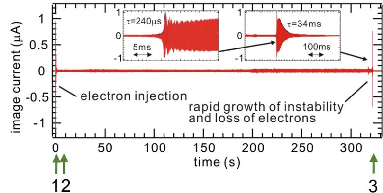
Selective decay of turbulence and spontaneous creation of stable vortex structure that lasts for more than 300s.
