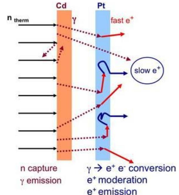
Positrons are generated by pair production from absorption of high-energy prompt gamma-rays after thermal neutron capture in Cd
