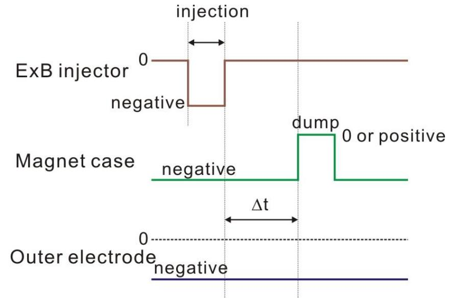
Injection, trap, and dump cycle
