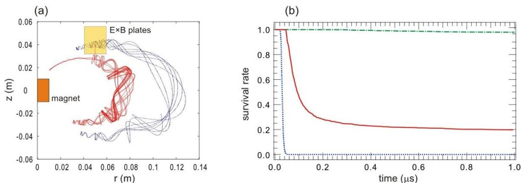
**Figure 3.** (a) Typical positron orbit projected onto the  $r$ - $z$  cross section when the electric field is applied (solid line) and not applied (dot line). Electric field of  $E = 1 \times 10^3$  V/m was applied in the marked region from  $t=0$  to  $0.1 \mu\text{s}$ . (b) Ratios of remaining positrons after injection without  $E$  (dot line), with the application of  $E$  (solid line), and when the magnet was also biased (chain line).
