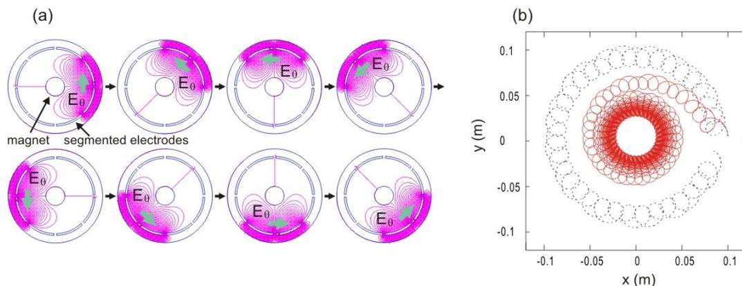
**Figure 4.** (a) Schematic view of a rotating wall and equipotential contours generated by the segmented electrodes. (b) Typical positron orbits with (dot line) and without (solid line) the rotating wall.
