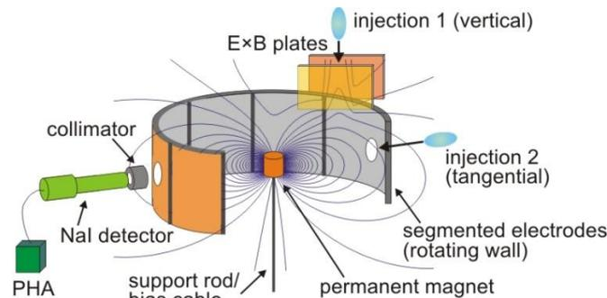
**Figure 2.** Schematic drawing of a proof-of-principle experiment, including the supported neodymium magnet,  $E \times B$  plates for vertical injection, rotating wall for tangential injection, and diagnostics.
