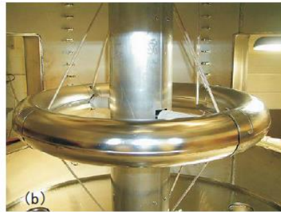
Potential control by using torus electrodes
