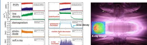
Visible light and x-ray image of plasma generated by ECH at 2.45GHz
