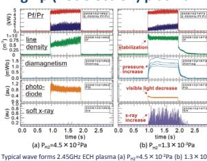
Typical wave forms 2.45GHz ECH plasma (a)  $P_{\text{ECH}} = 4.5 \times 10^{10} \text{ Pa}$  (b)  $1.3 \times 10^{10} \text{ Pa}$ .
