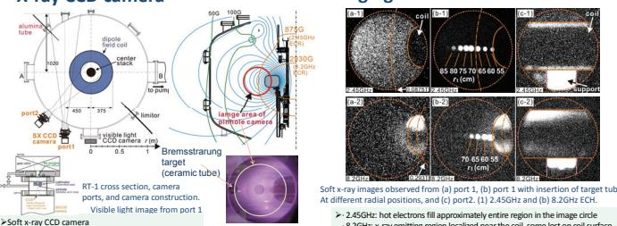
Soft x-ray images observed from (a) port 1, (b) port 1 with insertion of target region at different radial positions, and (c) port 2. (1) 2.45GHz and (2) 8.2GHz ECH.
