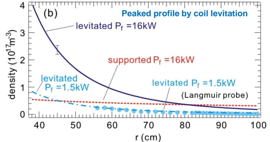
Radial density profiles [coefficient  $a$  of  $n(r)=n_0 r^a$ ] with and without coil levitation
