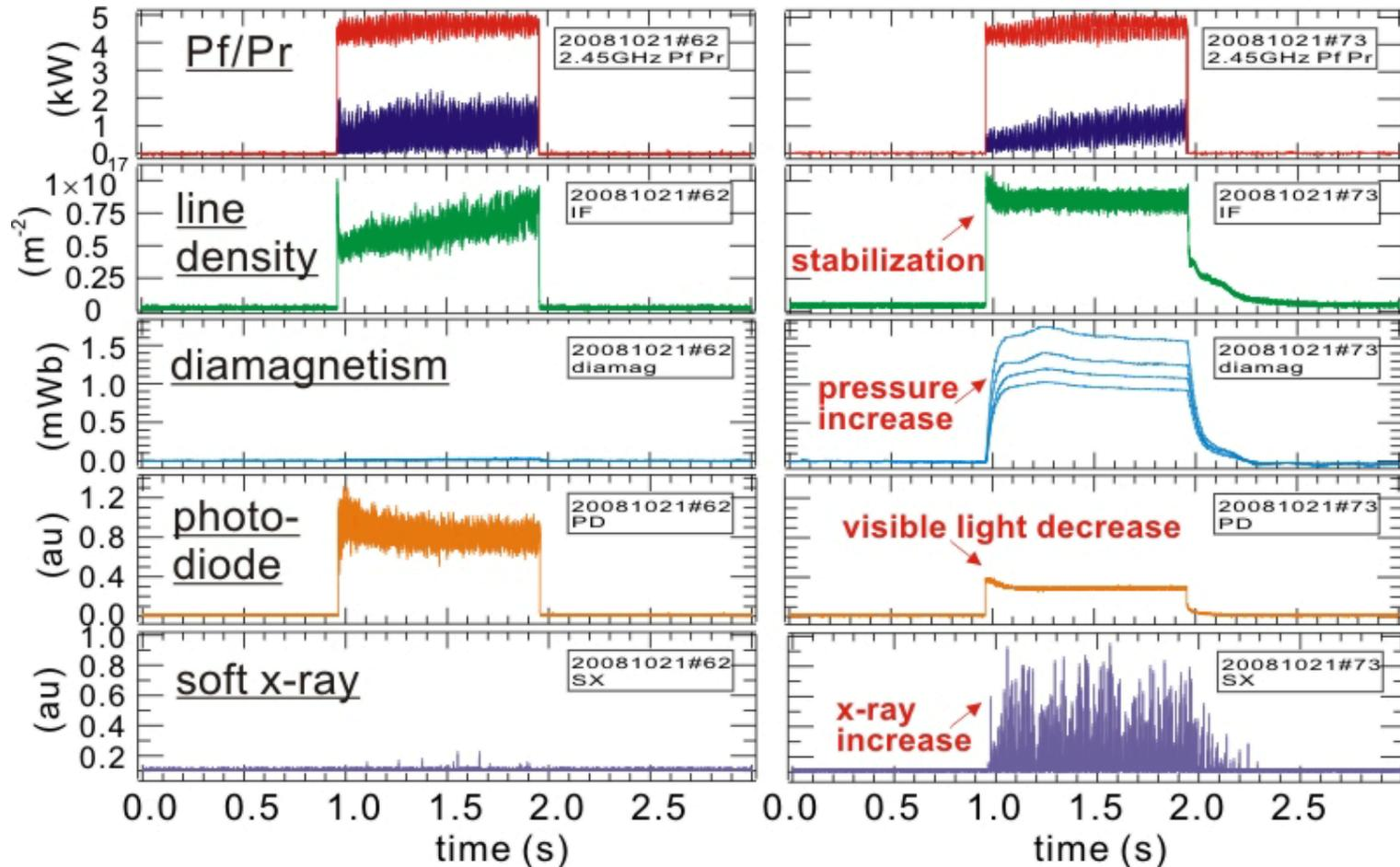
Waveforms of ECH plasma in RT-1 with (a)  $P_{H_2} = 4.5 \times 10^{-2} \text{ Pa}$  (b)  $1.3 \times 10^{-3} \text{ Pa}$ .
