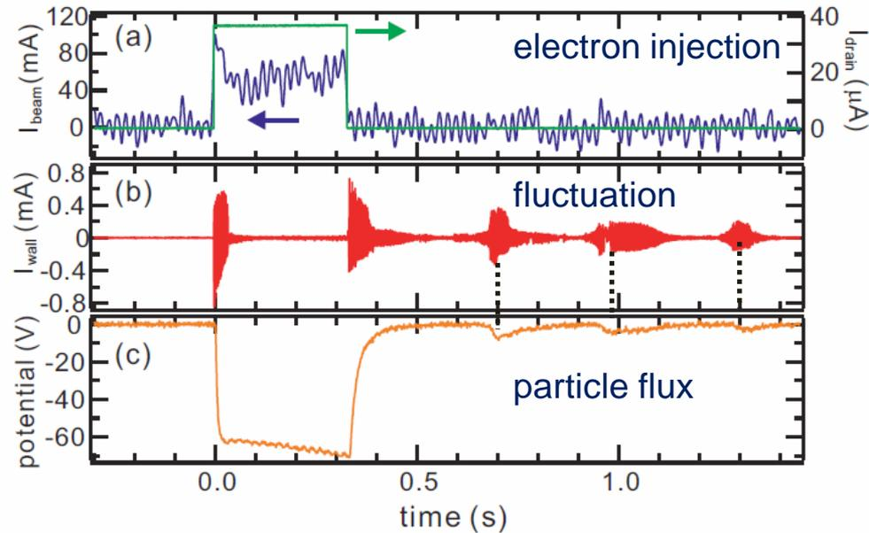
Onset of instability and particle flux at different magnetic surface
