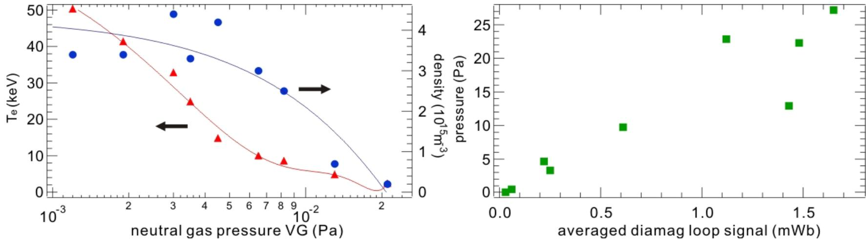
Temperature and density of hot electrons in variation of filled neutral gas, and hot electron pressure  $P_h = n_h T_h$  in variation of diamagnetic signal.
