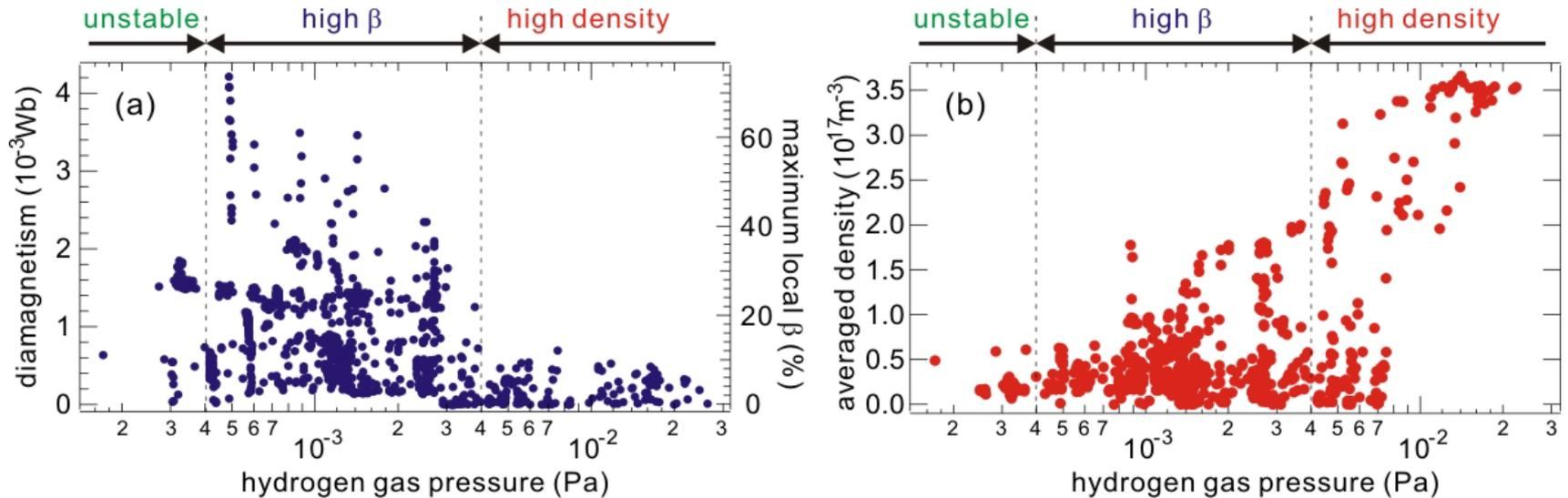
Diamagnetic signal (with calculated maximum local  $\beta$ ) and line averaged density
