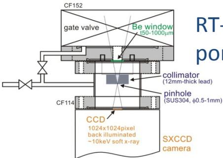
RT-1 cross section, camera ports, and camera construction.
