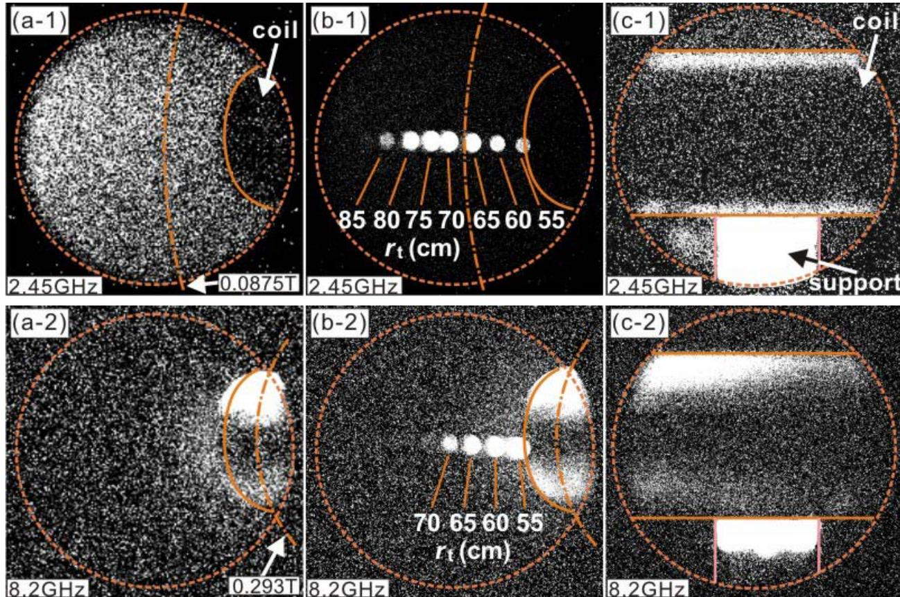
Soft x-ray images observed from (a) port 1, (b) port 1 with insertion of target tube at different radial positions, and (c) port2. (1) 2.45GHz and (b) 8.2GHz ECH.
