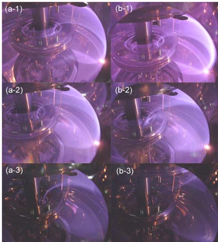
Visualized electron beam orbits agree with shape of magnetic surfaces.
