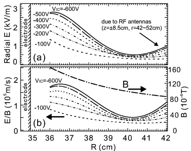
FIG. 7. The profiles of (a) radial electric field strength and (b) poloidal magnetic field strength  $B$  and  $\mathbf{E} \times \mathbf{B}$  drift speed at  $z=0$ , when the electrode bias voltage was modified from  $V_{IC} = -600$  V to  $-100$  V, calculated from the potential distribution in Fig. 5.
