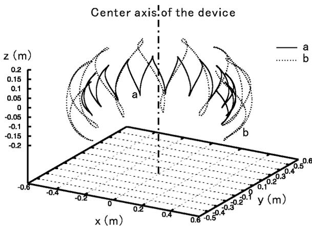
FIG. 2. Hydrogen ion orbits in the radial electric field and poloidal magnetic field of the Proto-RT. The initial position of the ion is (a)  $r=0.4 \text{ m}$ ,  $z=0.1 \text{ m}$  and (a)  $r=0.4 \text{ m}$ ,  $z=0.2 \text{ m}$ , respectively. Charged particles undergo toroidal  $\mathbf{E} \times \mathbf{B}$  motion and reflection motion due to magnetic mirror effects.
