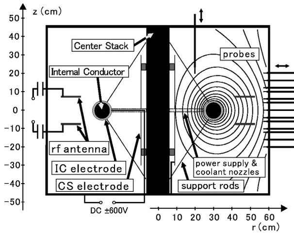
FIG. 1. Poloidal cross section of the Proto-RT chamber and magnetic surfaces of the poloidal field configuration. A pair of vertical field coils are located outside of the chamber (not seen). rf terminals are connected to a 13.56 MHz power source via dc cut capacitors and a matching circuit.
