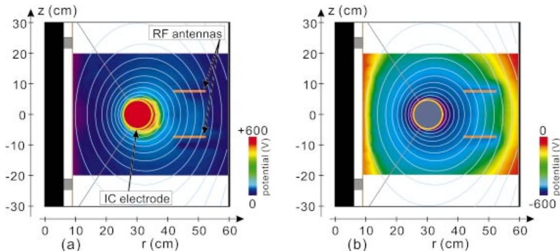
FIG. 6. (Color) Potential distribution of plasmas in the poloidal cross section of the Proto-RT, (a) when the IC electrode was positively biased ( $V_{IC} = +600$  V), and (b) negatively biased ( $V_{IC} = -600$  V). Thin lines show the poloidal magnetic surfaces.
