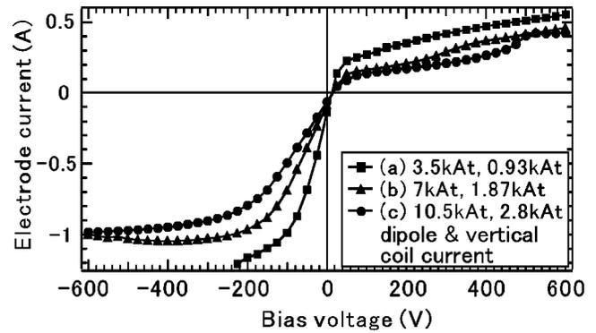
FIG. 3. Applied voltage on the IC electrode vs current between the electrode and chamber wall.
