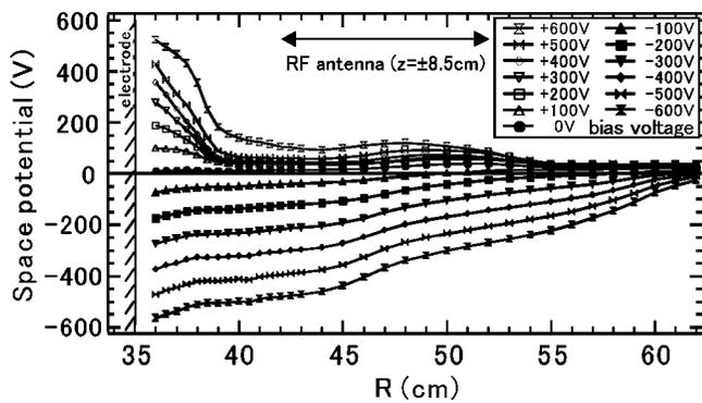
FIG. 5. Radial potential profiles (floating potentials of emissive Langmuir probes) of plasmas at  $z=0$ , with an IC electrode bias voltage of  $V_{IC}$  from  $-600$  to  $+600$  V.
