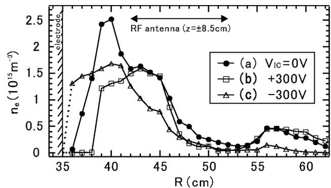
FIG. 4. Radial profiles of electron number density at  $z=0$ , (a) when  $V_{IC} = 0$ , the electrode is grounded, (b) positively biased  $V_{IC} = +300 \text{ V}$ , and (c) negatively biased  $V_{IC} = -300 \text{ V}$ .
